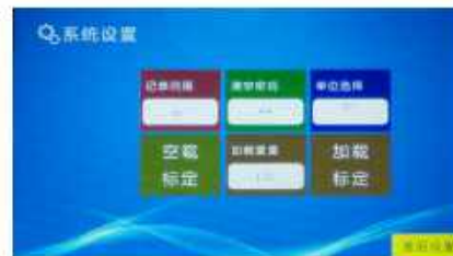
Weight set system including the timer, password, unit, weight data with loading or without loading
